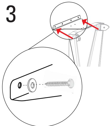
**EN** Starting at the universal bracket drill a  $\frac{1}{4}$ " diameter hole 2" deep at each mark. Assemble a washer on a lag screw and screw into each hole until tight.
