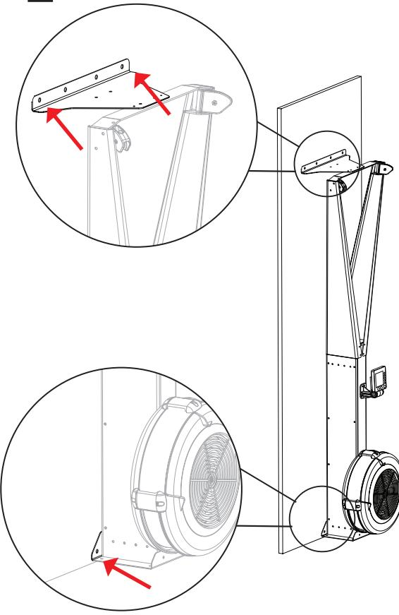
**EN** Hold the SkiErg up against the wall. The two outside holes on the universal bracket should be lined up with the wall studs. Mark each hole location. Also mark each hole location where the SkiErg bottom bracket lines up with the wall (left and right side).
