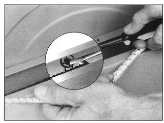
Press on the new Tuflok screw head to expand its base and attach the pickup to the frame.
