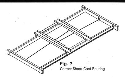
The enclosed parts were designed in response to Slide bungee cord wear problems noted in the field. Use of these components is optional but recommended on older slide units where the cord is looped around the Slide Base and routed through two holes in the Slide Carriage.
